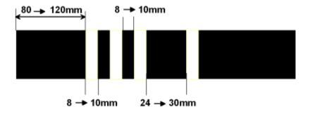
**(a).** Distance between the bars Group 1 and 2: minimum 24mm and maximum 30mm
